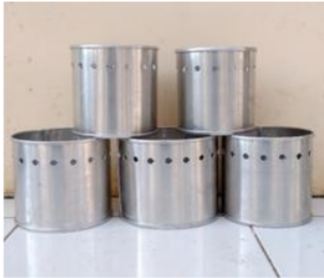
Figure 1. The shell of burning chamber
